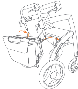
Figure 30: Attaching the transport chair package.
